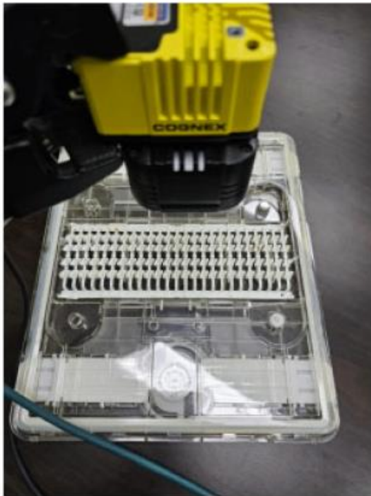
Capable Profile Inspection with IS3800 Easy Deep Running as well Gap Measurement
